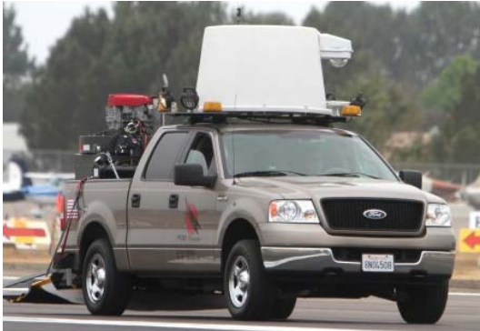
Trex FOD Finder™ XM is a mobile FOD detection and retrieval system designed for runway, taxiway and apron operation. XM can be operated at driving speeds up to 50 Km per hour.
